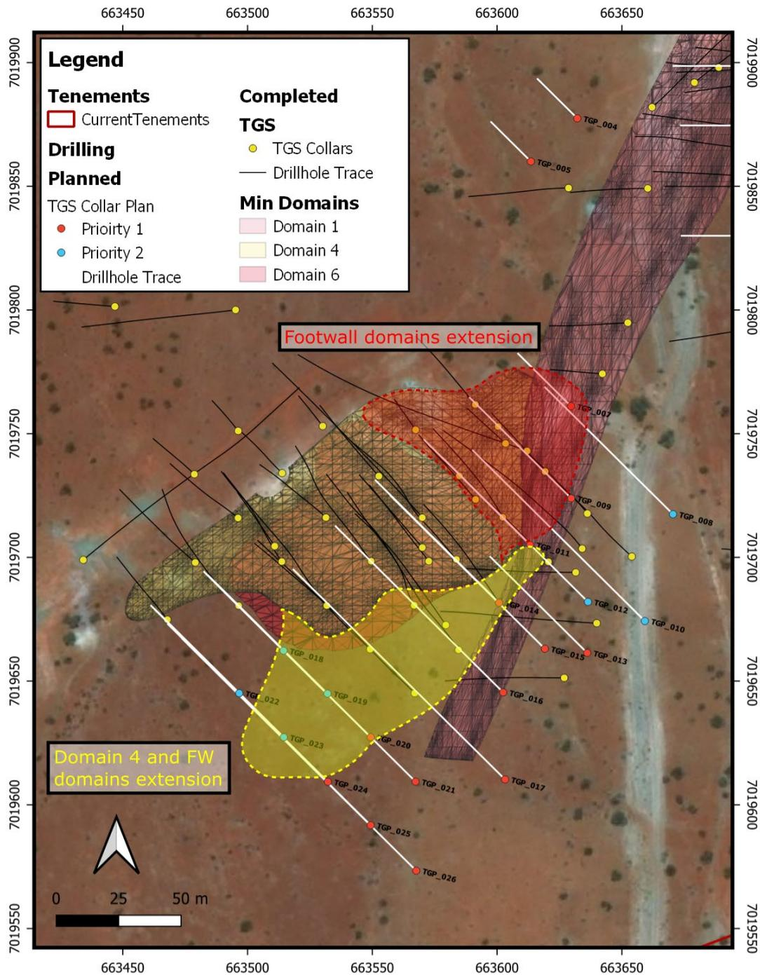
**Figure 1 Tumblegum South Project Proposed new drilling**
